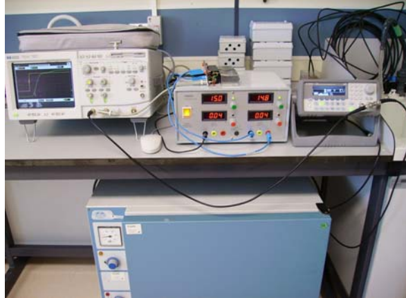
Fig. 3.5 Experimental set-up for measurements of transient responses: Faraday cage (down), wave generator (up-right), amplifier with power source (up-centre), and oscilloscope (up-left)
