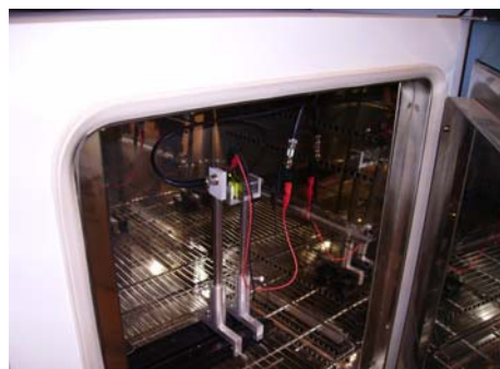
Fig. 3.3 Electroluminescence equipment for electro-optical measurements in organic-based devices: Integrating sphere (left-hand side) and Faraday cage (right-hand side), respectively.
