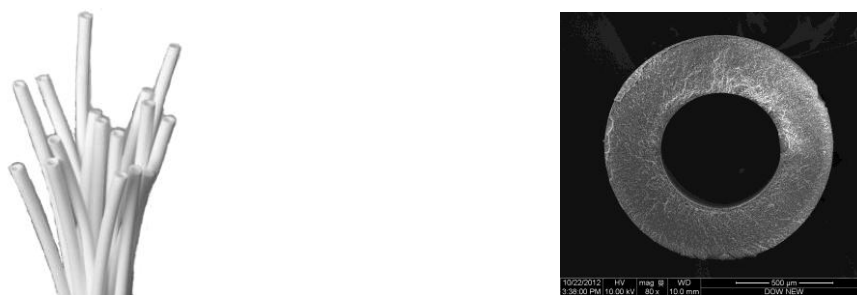
Figure 5. PVDF hollow fibers and its section
