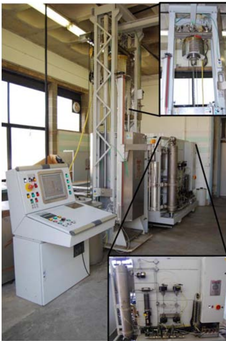
Figure 10. HPP unit Model ISO-LAB FPJ 11500 from Stansted Fluid Power Ltd., Essex, UK
