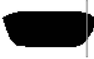
Figure 4.5: Bubble being detected by a rectangular AOI with a length of 1 pixel.
