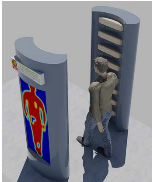
Figure 1.3: Artist view of a passive scanner portal that is capable to detect objects concealed beneath the clothes. The working principle of this portal is to distribute in a vertical disposition a group of horizontal passive arrays in such a way that a 2D image is obtained.
