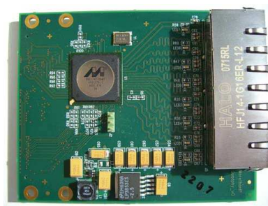
Fig. 6. 4 - Ethernet interface modules for UNI: HSMC 4-Ports 10/100/1000Base-T RJ-45 port Adapter Board
