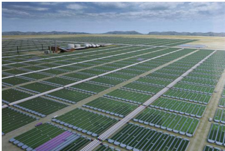
Figure 3 Algae open pond farm for biofuel and jet fuel production ( http://www.petrosuninc.com )
