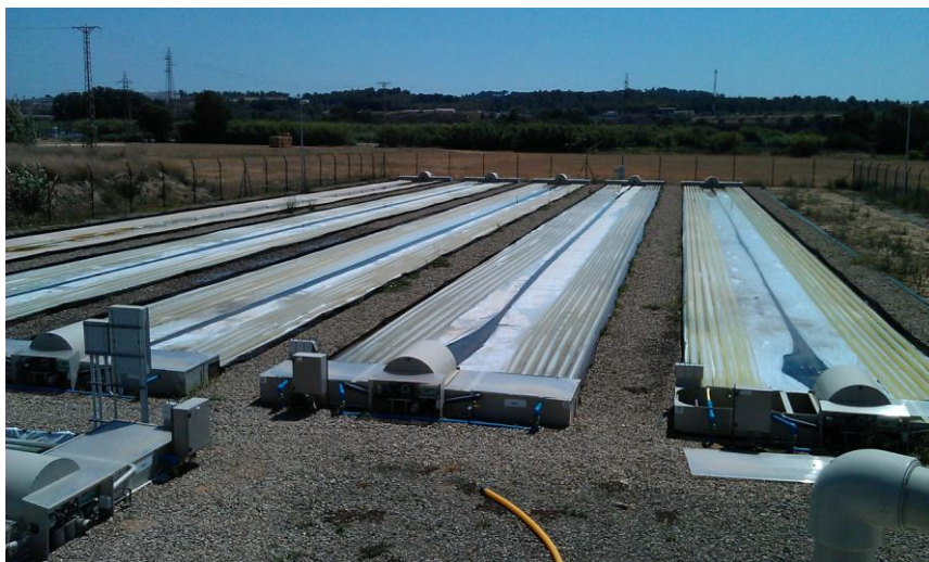
Figure 4 Tubular Photobioreactors for microalgae production (Pilot Plant-Repsol, Tarragona)
