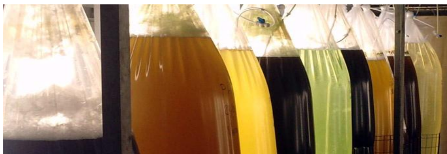
Figure 1 Vertical tubular 300L fotobiorreactors from different microalgae species tested in this work. Phaeodactylum tricornutum , Nannochloropsis gaditana and Chaetoceros calcitrans .
