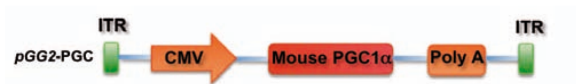
Figure 19. Schematic representation of the construct used to produce the AAV-PGC vector. CMV: cytomegalovirus promoter; poly A: Simian Virus 40 Polyadenylation signal; ITR: Inverted terminal repeat.
