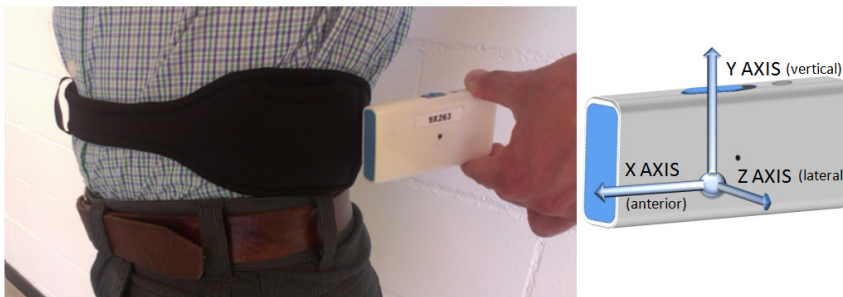
Figure 3.1: Movement sensor used and its position in a neoprene belt.
