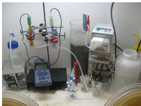
Figure 3. Set-up of the flow-through experiments. Flow rate in the experiment was controlled by a peristaltic pump. Arrows indicate the flow direction in the flow-through experiment.
