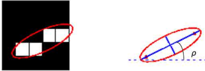
Figure 3.30: Orientation of a cluster. Red line: defined ellipse, blue lines: axes. [Taken from documentation of Imaging Processing Toolbox of Matlab®]
