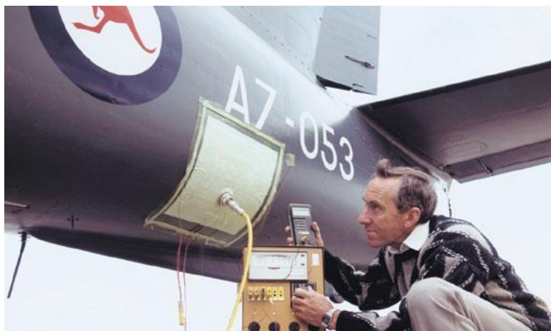
Figure 1.1 On-site structural repair of an aeroplane
