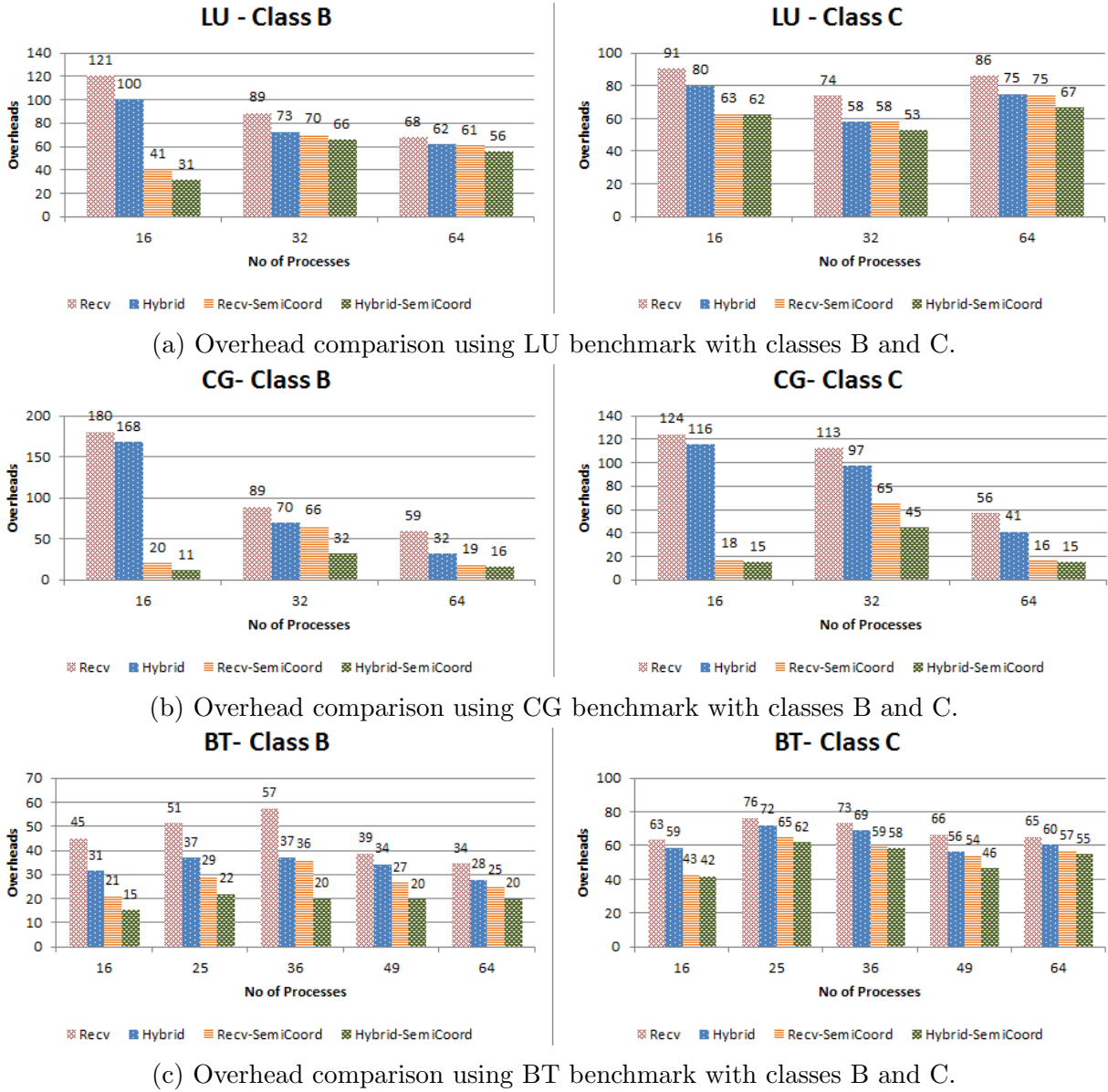
Figure 6.3: Comparison of overheads using the Hybrid Message Pessimistic Logging and the Pessimistic RBML considering the NAS Parallel Benchmarks.
