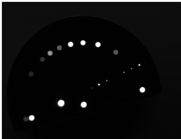
Fig. 3.8 A picture of the probe tip. Since the illuminated light to different fibers was not homogeneous they have different brightness. The smaller dots correspond to single mode fibers (DCS detector fibers).
