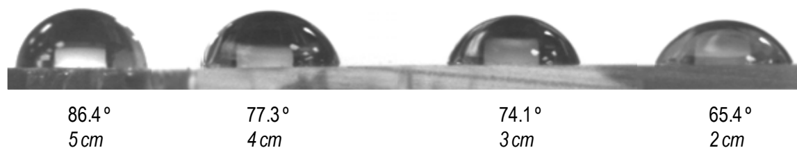
Figure 57. Water contact angle in photo-chemically modified glass surface dependence on height.
