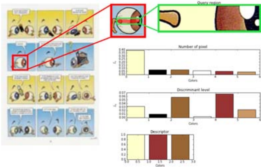
Figure 4.13: The left part represents a query example after the colour reduction process and its original image. Top-right part shows the colour histogram of the 6 first colours with the highest number of pixels in the query as a percentage from the total number of pixels in the query ( L_1 ). Middle-right figure represents the corresponding discriminability level for each colour according to the other pixel in the page. Bottom-right figure represents the corresponding query descriptor of N = 3 colours. Image credits: [86].
