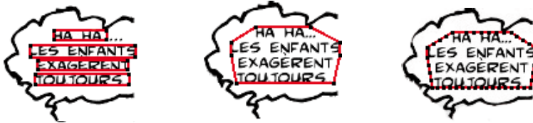
a) Group of text lines b) Text area convex hull c) Snake initialization
