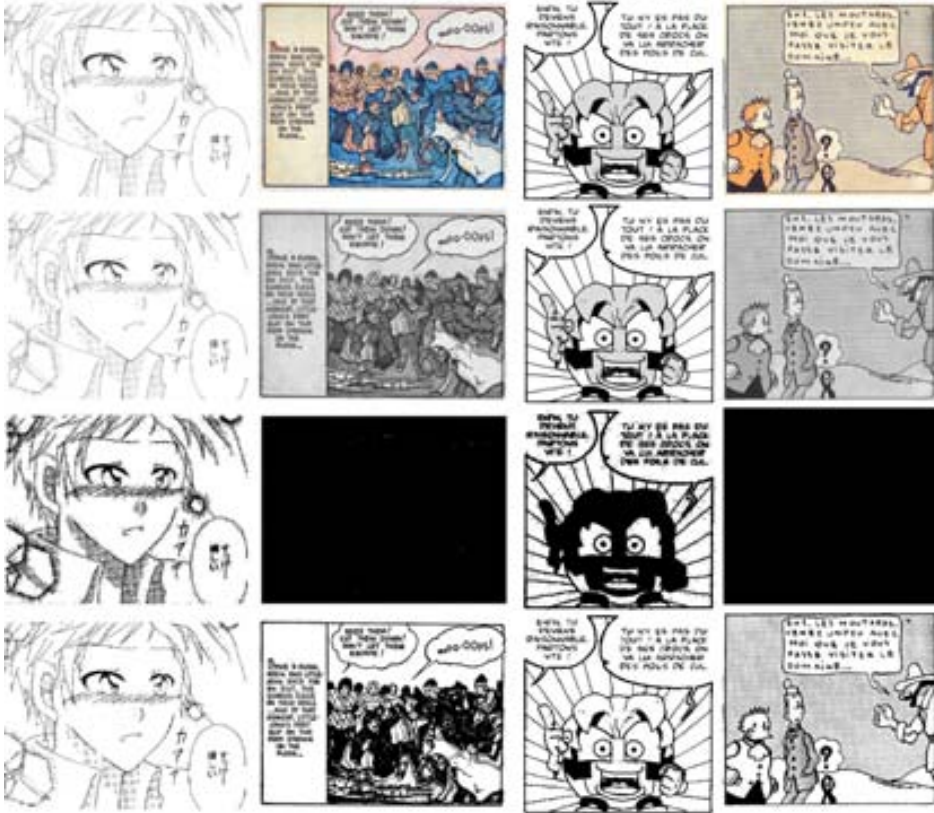
Figure 4.2: Different threshold selection methods applied on the luminance channel of several comics types. First row shows the original image of a selection of comic book parts. Second row shows the corresponding luminance channel of HSL colour space in a 8 bits grey-scale image. The third row represents the bi-level segmentation of the grey-scale image with a fixed threshold at 250 (as Arai [7]) and the fourth row shows the corresponding results using the automatic Otsu's threshold selection method. Image credits: [35, 68, 106, 123].
