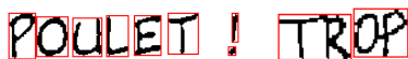
Figure 4.3: Example of connection between connected components. On the left, a word with six well separated letters, on the right a word detected as two pairs of attached letters because of the handwriting variability and segmentation process.
