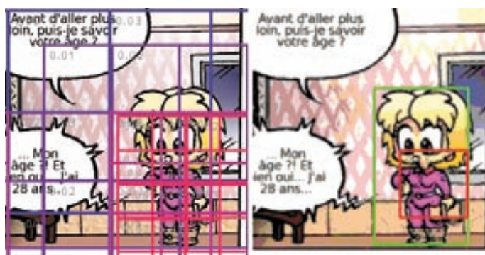
Figure 4.15: Multi-scale spotting example. The left image shows the detections at different scales, the colouration depends on to the p value, blue to red for low to high. The right side image shows the remaining best detection after the filtering step. Image credits: [34].
