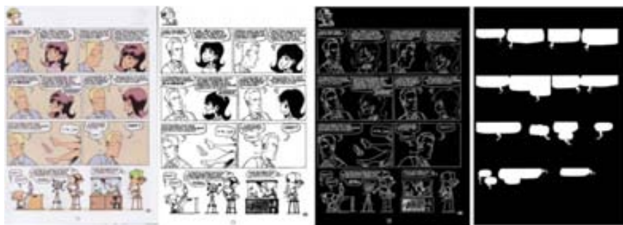
Figure 4.6: Balloon extraction process. Original image, binary segmentation, contour detection (connected components) and result mask from left to right. Image credits: [115].
