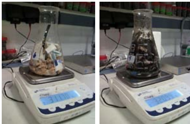
Figure 4.1. SSF starts at laboratory scale. Preparing samples of soy fiber residues (left) and coffee husk (right) for respirometric assay.
