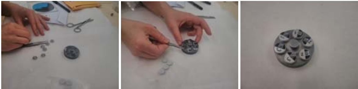
Figure 3.12 Preparation of liquid samples for the observation by SEM.
