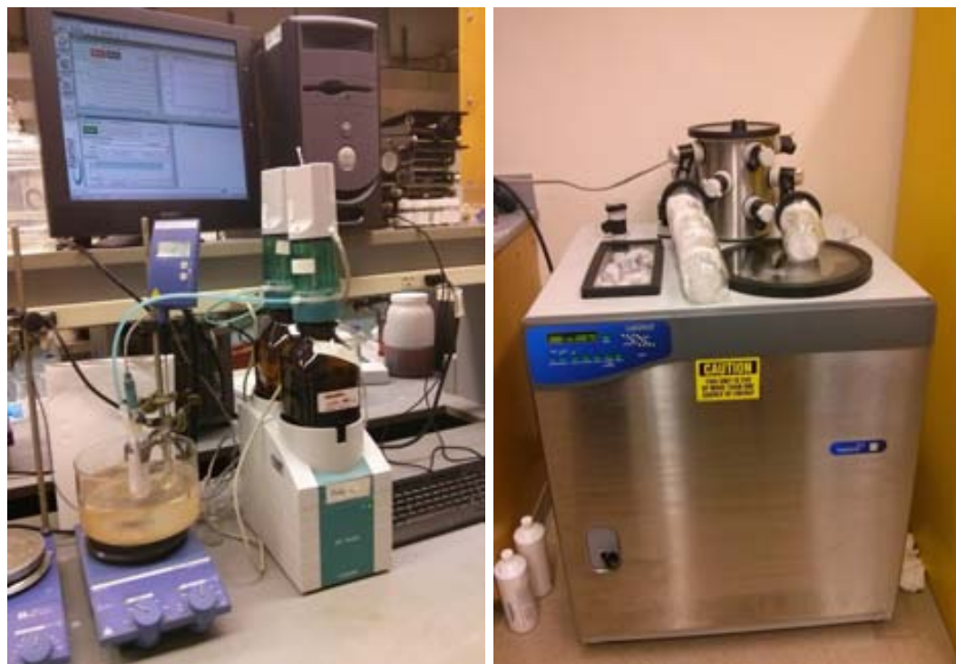
Figure 8.3. Hardware and Software Instruments used for Proteases catalyzed synthesis reactions (left) and lyophilizer machine (right) at RPI.
