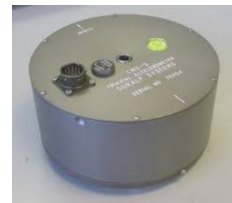
Figure 2.7. Left: the general force feedback control system (Stuart-Watson, 2006). Right: CMG-5T feedback accelerometer ( www.guralp.com ).
