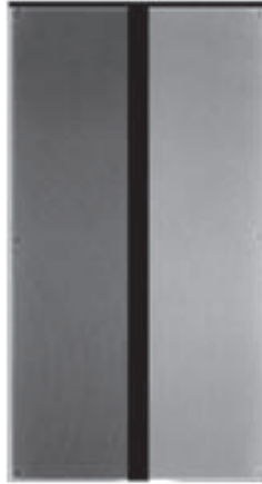
Figure A.4: Flat exposure with a light level of \sim 27.000e^- . The serial register is divided in two and in this image the serial overscan is displayed on the center of the CCD. The parallel overscan is displayed on the top of the image (Estrada et al. (2010)).
