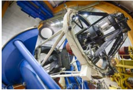
Figure 4.2: The Dark Energy Camera, mounted on the Blanco telescope at the Cerro Tololo Inter-American Observatory in Chile. Credit: Reidar Hahn/Fermilab.
