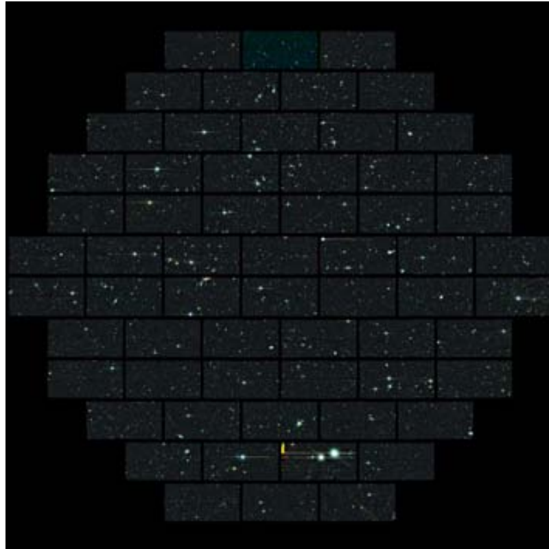
Figure 4.7: Composite Dark Energy Camera image of one of the sky regions that the collaboration will use to study supernovae, exploding stars that will help uncover the nature of dark energy. The outlines of each of the 62 charge-coupled devices can be seen. This picture spans 2 degrees across on the sky and contains 520 megapixels.
