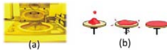
Fig A.18. (a) Photo of the machine used for spin coating (called “spinner”); (b) Sketch of the spin coating procedure used as a first step in the lithographic process.
