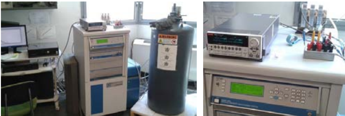
Fig A.15. Photo of the Physical Properties Measurement System (PPMS) at the ICMAB, configured to use the external Keithley as source.
