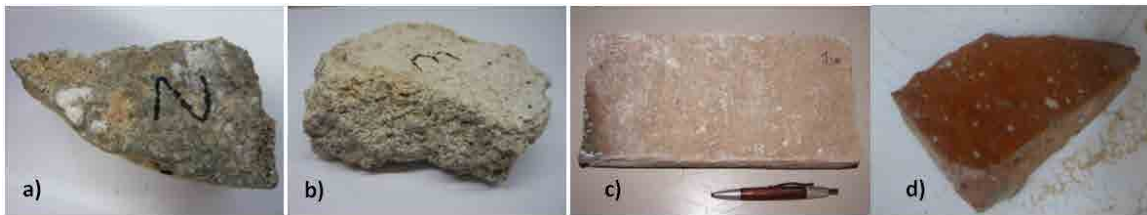
Figure 2.6. Photographs of (a) fragment of cement mortar used in columns, (b) fragment of lime mortar used in walls, (c) clay brick used in walls, and (d) fragment of clay brick used in columns.
