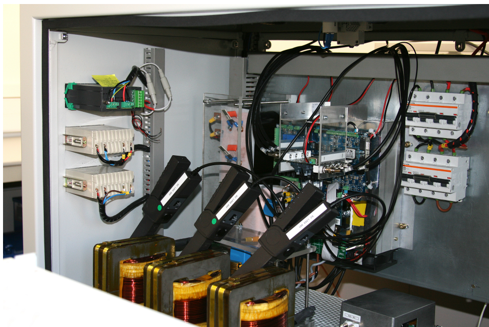
Fig. A.5: Three phase interleaved dc-dc converter
