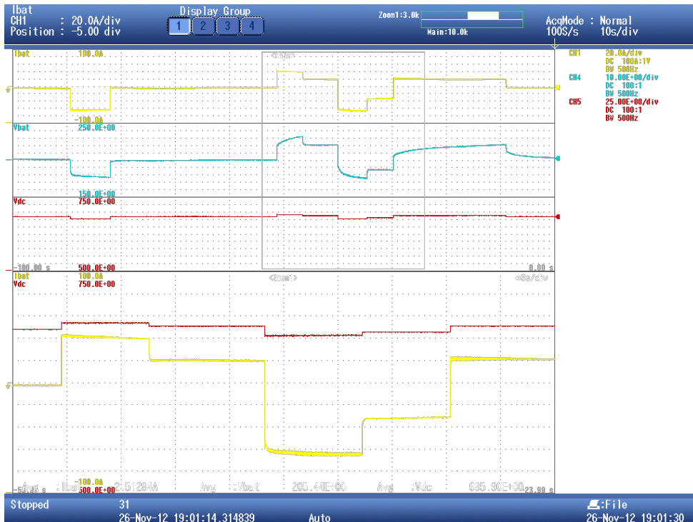
Fig. A.9: Droop voltage control. Total battery current (yellow), battery voltage (cyan), dc bus voltage (red)
