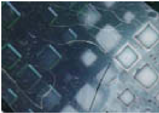
Figure 49 - Non-homogenous bonding and invasion of the PCR chambers by Mylar film.
