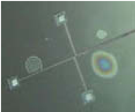
Figure 50 - Electrophoresis cross-injection chip with bonding anomalies. Micrometer impurities lead to millimeter non-bonded areas.
