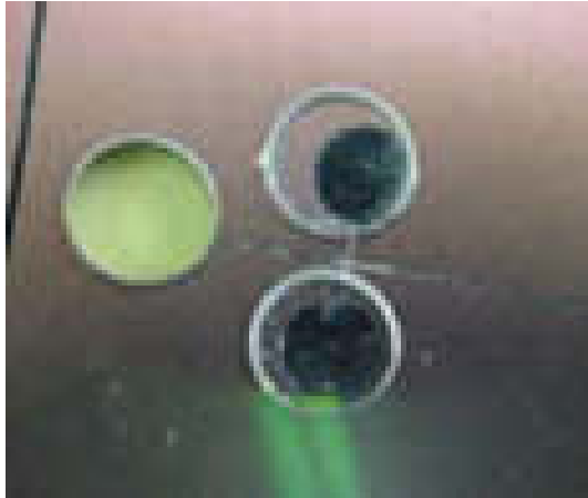
Figure 51 - Electrophoresis cross-injection chip with two correctly drilled holes and a badly timed hole that perforates the silicon substrate. Stuck abrasive debris can be seen as clearer areas in the channel structure.
