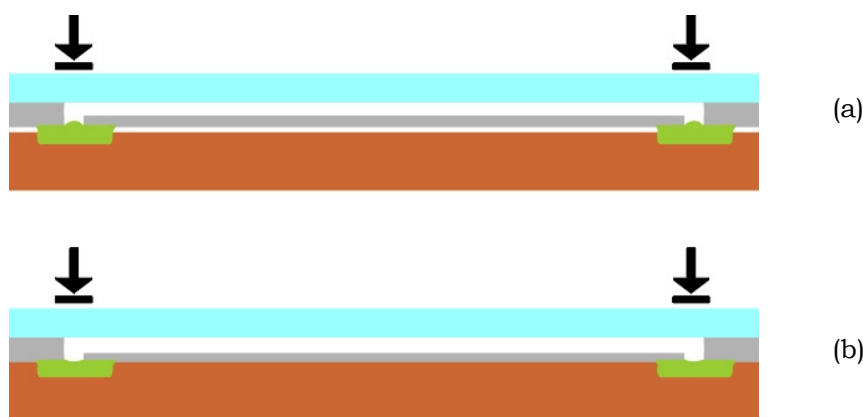
Figure 95 - Sealing with rubber gaskets and problems arising from under-drilling (a) or over-drilling (b) of the gasket hole.
