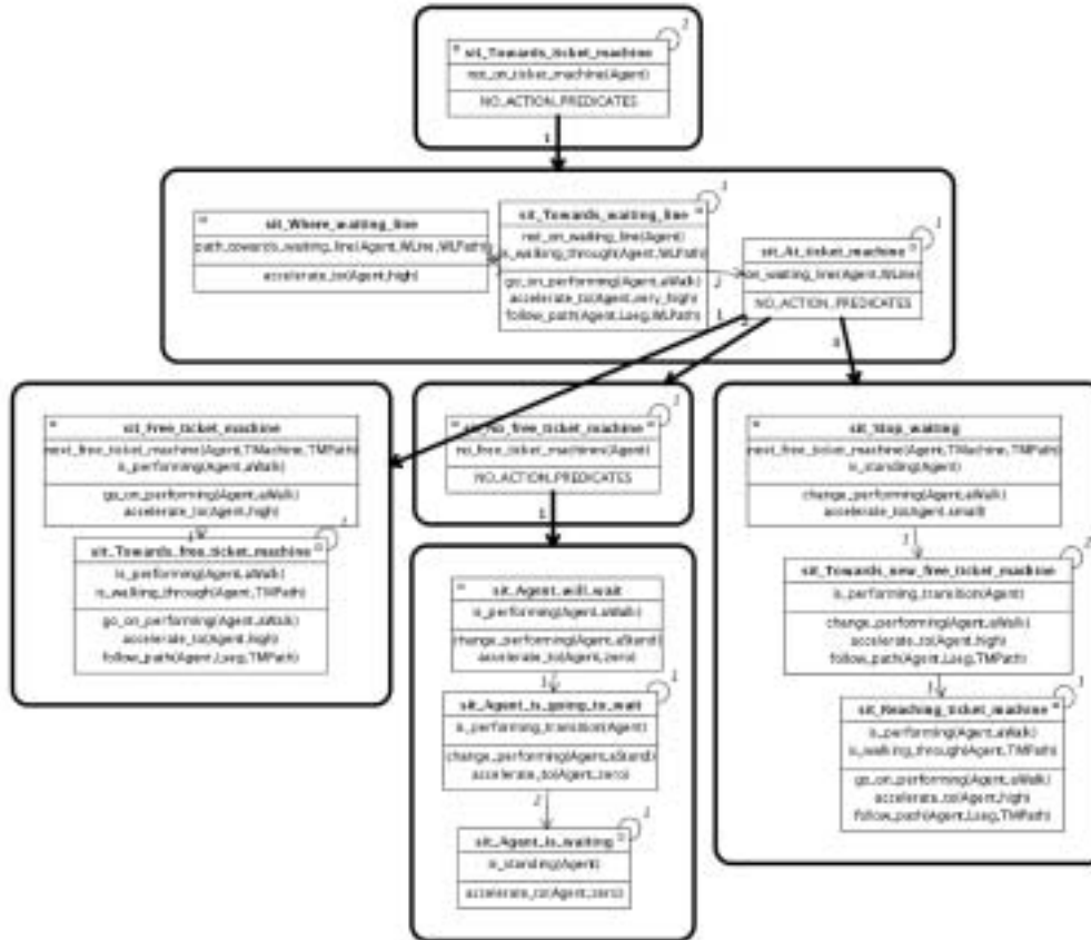
Figure 5.10: Automatic generation of a synthetic behavior: the situation scheme called sit_Towards_ticket_machine .
