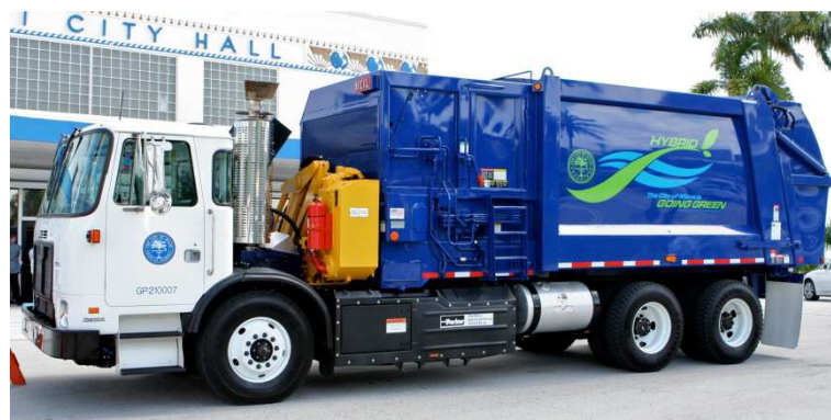
Fig 12. Autocar RCV equipped with a Parker Runwise system
