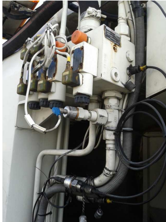
Fig. 22. Detail of the datalogging system, pressure values acquisition
