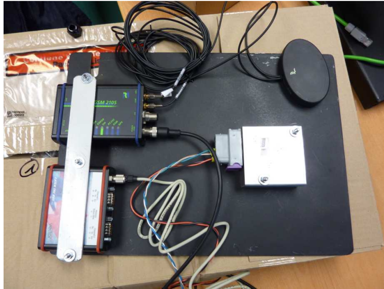
Fig. 19. Detail of the datalogging system for installation in the RCV cabin
