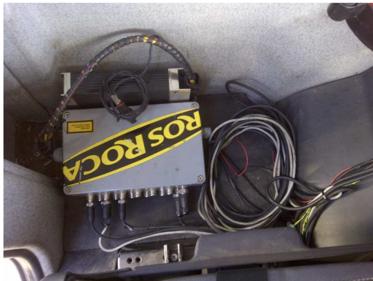
Fig. 20. Detail of the datalogging system for installation in the RCV cabin
