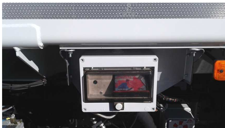
Fig. 21. Detail of the datalogging system for installation below the body
