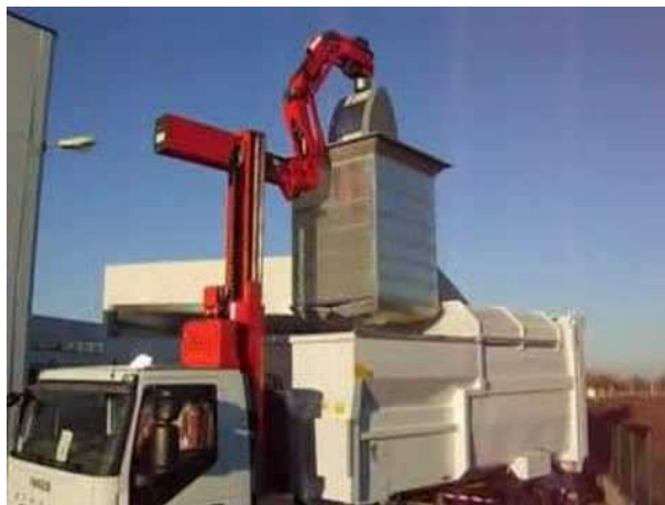
Fig 4. Bilateral side loader RCV
