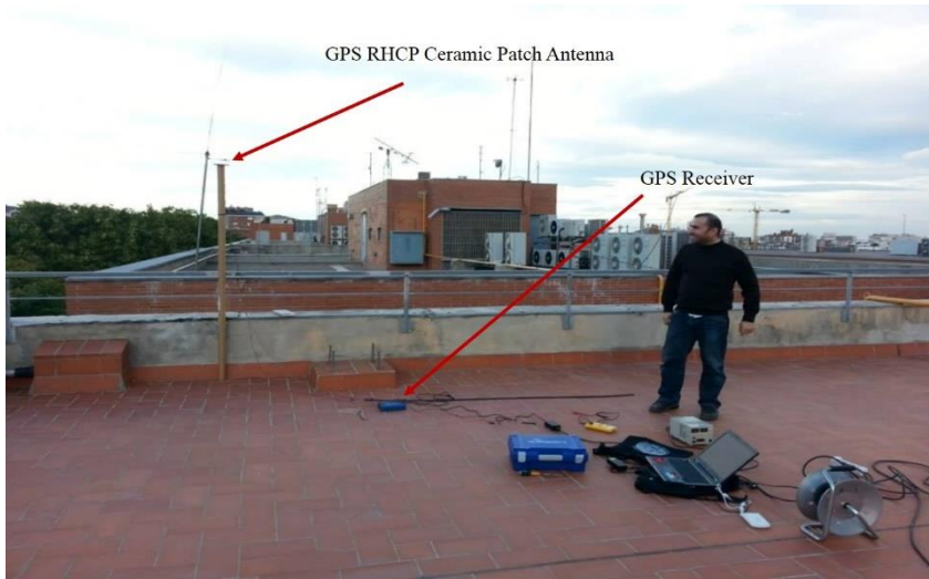
Figure B.1 Recording direct GPS signal process using GPS patch ceramic Antenna and Microwave amplifier (LNA), receiver and relevant equipments.
