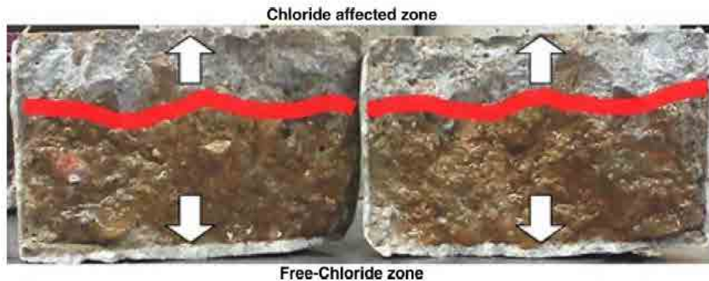
Figure 6.1: Chloride penetration depth by \text{AgNO}_3 solution spraying
