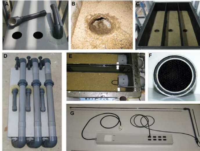
Fig. 2.2 - Different working phases during the construction of the actograph. A: the simulated burrow during the gluing at the bottom of the tank (sand was previously glued inside the burrow); B: A particular of the burrow with glued sand; C: The view of one painted tank; D: Underside the tank with the external down pipe which connects two opposite sides of the tank. E: The pump placed inside the pipe. F: A close view of the diffuser placed in the opposite side of the pump. G: The resulting L shaped submersible lighting system with multiple alimentation apparatus. The dashed line indicates the transparent methyl metacrilate (MM) tube in which was inserted the LEDs strips. The black line represents the smaller PVC tube, containing the cables for LEDs' power supply.
