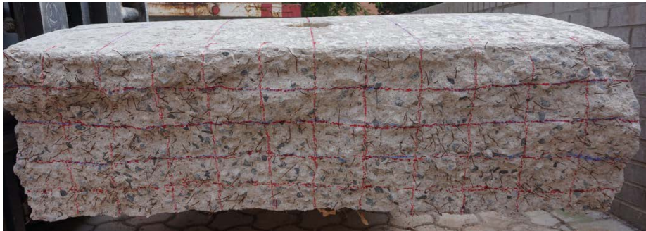
Figure 4.15 Grid generated to count the fibres in the fracture sections of the segments
