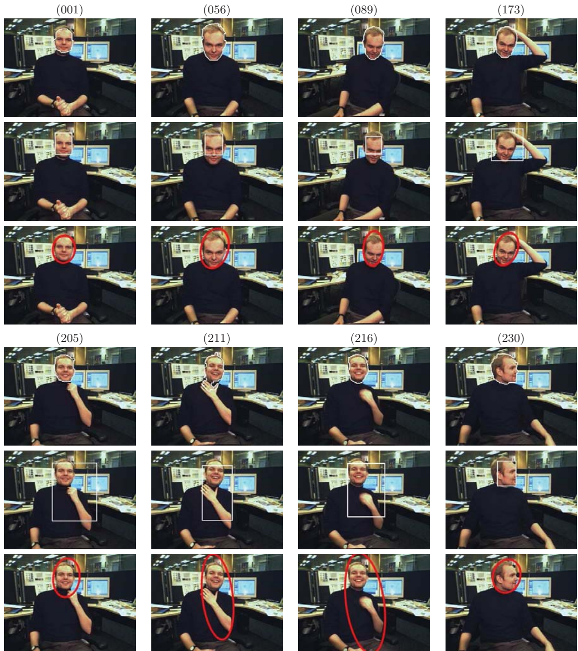
Figure 7.16: Results for 'Ms' sequence using region-based mean shift, ABCShift (rectangles) and Camshift (ellipses) algorithms.
