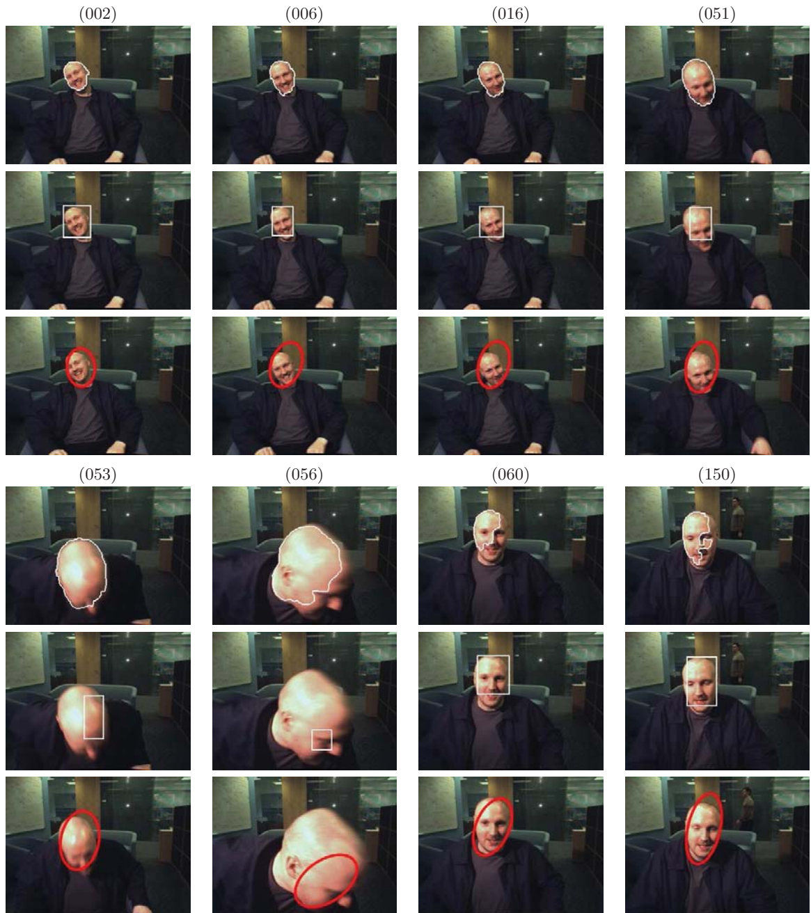
Figure 7.18: Results for 'Jm' sequence using region-based mean shift, ABCShift (rectangles) and Camshift (ellipses) algorithms.
