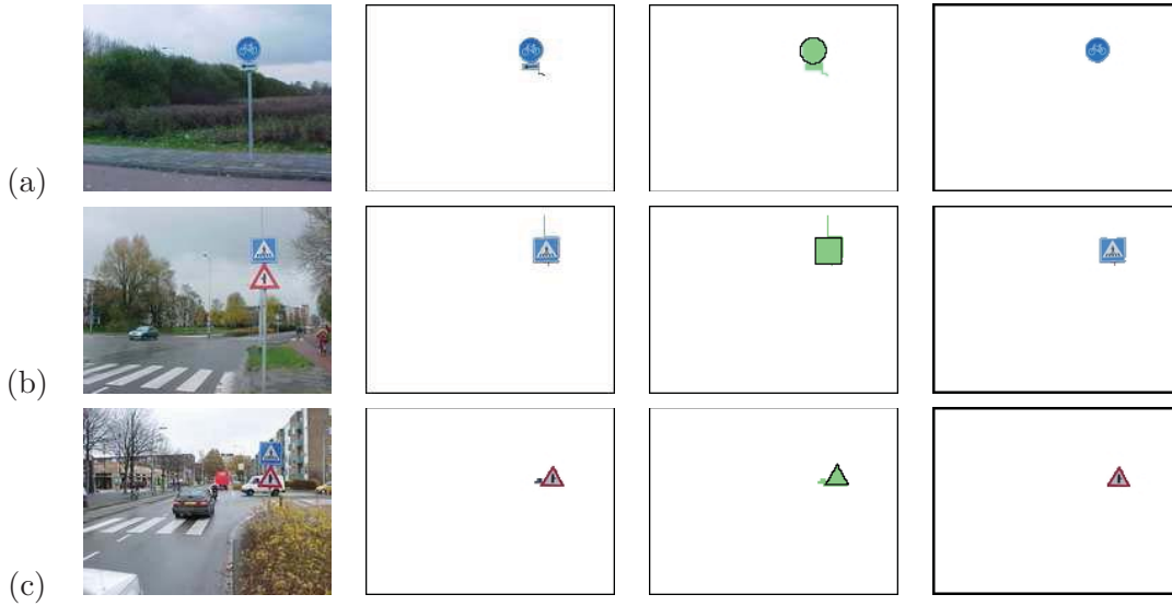
Figure E.1: Improvement in the representation of objects achieved by the extension of the nodes, for a traffic sign detection application. First column: original images. Second column: object nodes. Third column: shape fitting. Fourth column: extended nodes.
