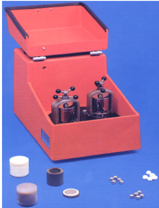
Figura 2.2: Photograph of the planetary mill used in the present work, a Fritsch Pulverisette 7 .
