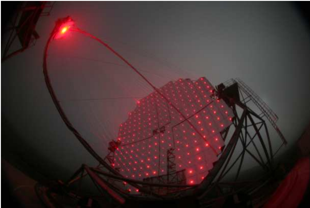
Figure 3.3: Mirror panel lasers switched on during re-alignment procedure. Not all mirror panels were installed at the time of the photograph.
