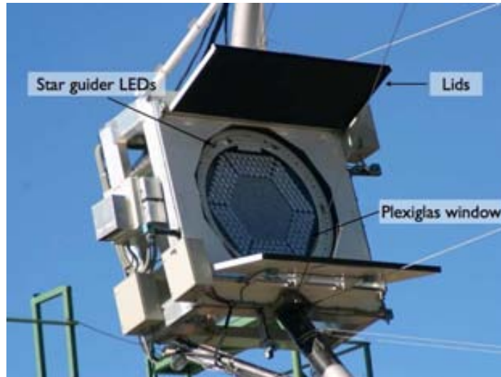
Figure 3.4: Front view of the MAGIC telescope camera. The plexiglas window protects the camera interior where the light concentrators collect the incident light onto the camera photosensors.
