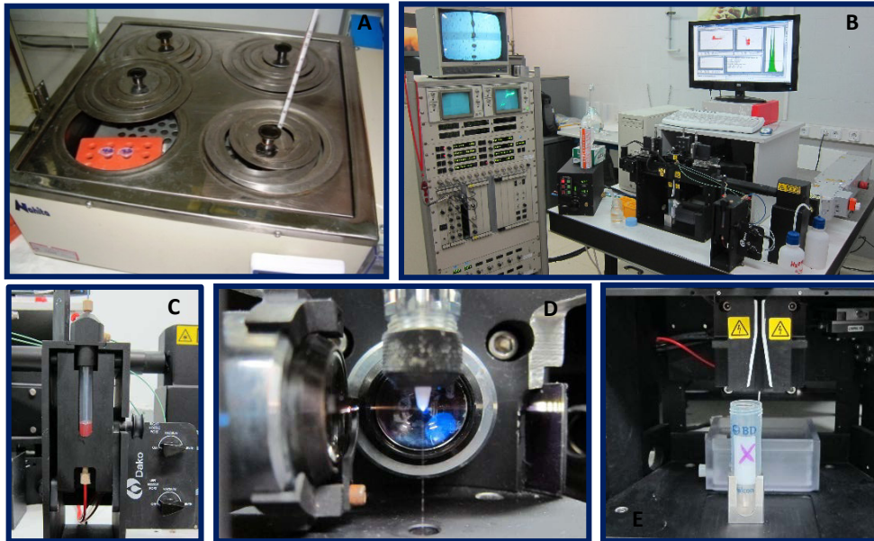
Figure 6. Flow cytometric sperm sex sorting. A: incubation of spermatozoa with H-42 in a water bath at 36 °C in the dark. B: MoFlo SX® flow cytometer/sperm sorter. C: sample stained with H-42 and FDA for sex sorting. D: ultraviolet laser impact on the sperm sample. E: charged deflection plates and X-chromosome-bearing sperm population collection.
