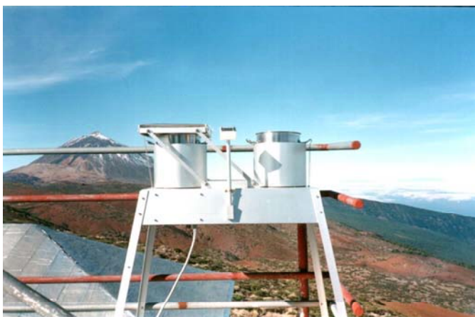
Figure 21. Deposition sampler at the Atmospheric Observatory of Izaña. On the background the peak of Teide is visible (Foto: Sandra Ribes)
