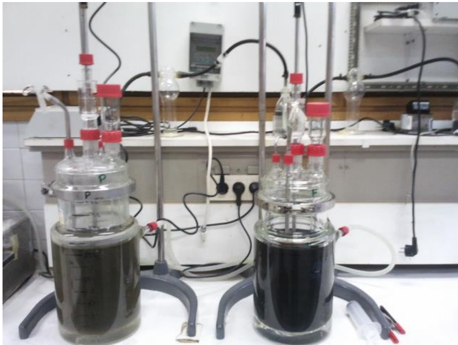
Figure 3.2 Laboratory semi-continuous stirred tank reactors used in UB
