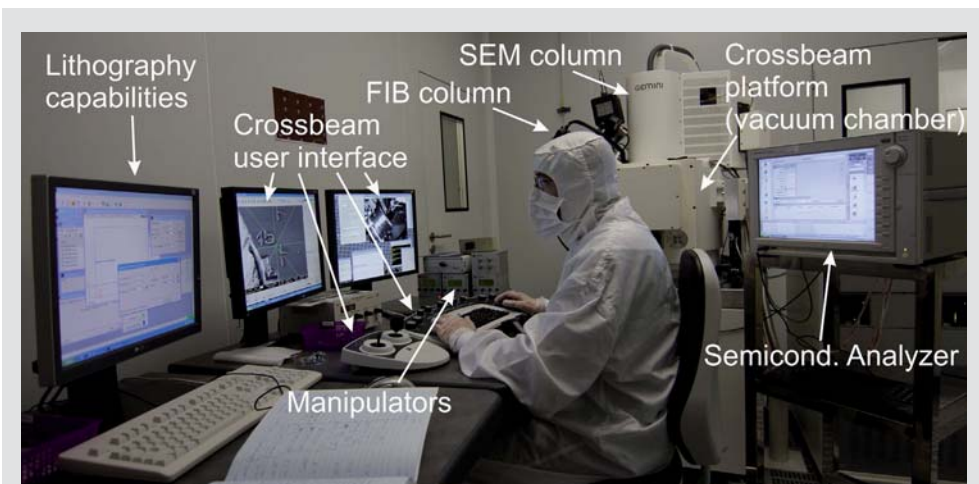
Figure 2. Photography of the Crossbeam used for the fabrication and characterization of the devices presented in this thesis. In the photography it is also observed some attachments connected to the Crossbeam, as the Elphy Quantum lithographic capabilities (Raith), three manipulators (Kleindiek) and a semiconductor analyzer (Agilent).
