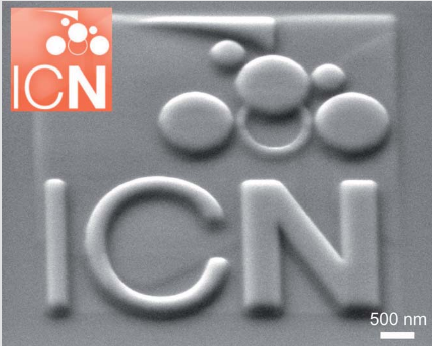
Figure 12. SEM image of a three dimensional pattern defined by FIBID deposition of Pt onto a silicon chip. The pattern has been generated from a grey scale picture the ICN logo.
