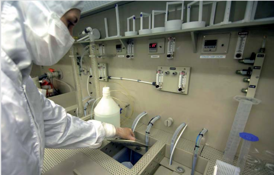
Figure 3. Photography of the chemical bench located in the Microsystems area of the ICTS Clean Room where the wet etching processes have been performed.
