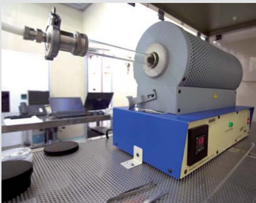
Figure 4. Photography of the CVD furnace (located in the Furnace area of the ICTS Clean Room) used to perform the high temperature diffusive boron doping of the devices.
