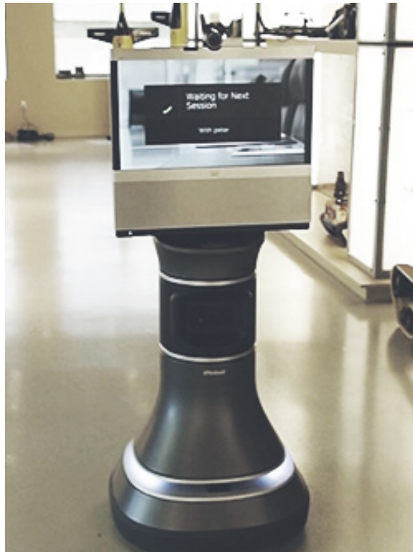
Figure 2.7: An image of the iRobot Ava 500, an autonomous roaming telepresence robot. Image taken from Wikimedia.org
