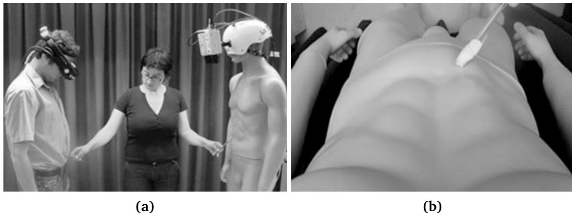
Figure 2.4: Experimental Setup of the Full Body Ownership Illusion study, as described by (Petkova & Ehrsson, 2008). In (a) the participant views the mannequin body from 1PP via the HMD when he looks down to see his own body, due to the cameras attached to the mannequin’s head. (b) The participant is given synchronous visuotactile stimulation by the experimenter to induce the full body ownership illusion over the mannequin. Images taken from (Petkova & Ehrsson, 2008).
