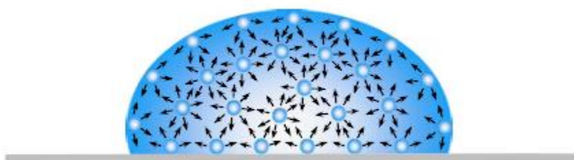
Figure 1.10: Surface tension is caused by the unbalanced forces of liquid molecules at the surface. (Taken from Surface Science Techniques , Springer Series in Surface Science 51, DOI: 10.1007/978-3-642-34243.1_1, 2013)
