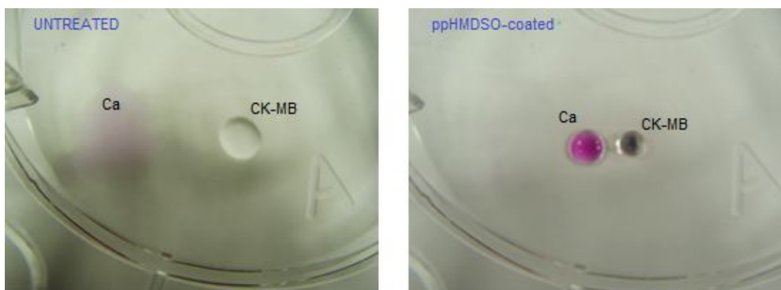
FIGURE 5.17. Assessment of the improvement in hydrophobic behavior of ppHMDSO-coated rotor (RIGHT) as compared to an untreated rotor (LEFT) by depositing 5\mu\text{L} of Ca and CK-MB reagents.
