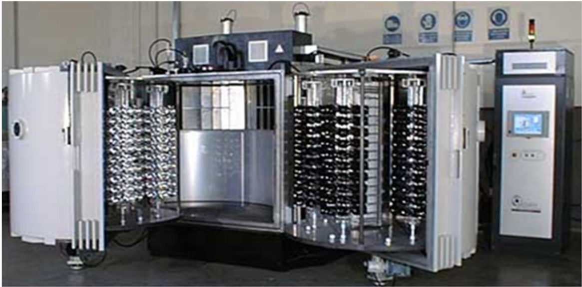
FIGURE 1.12. Commercial vacuum metallization and plasma polymerization reactor with a rotating planetary system for homogeneous coating deposition.
