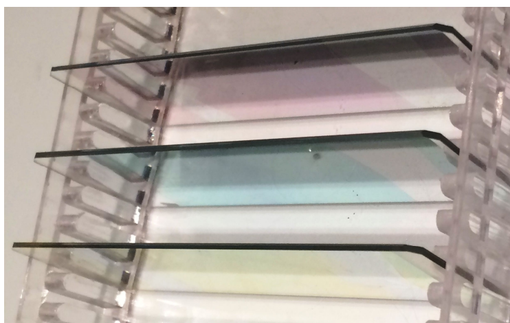
FIGURE 3.11. Films with homogeneous thickness deposited on a parallel-plate electrode configuration.
