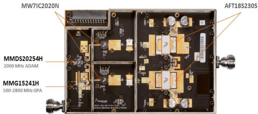
Figure 2.5 Cellular power amplifier reference design in [88]
