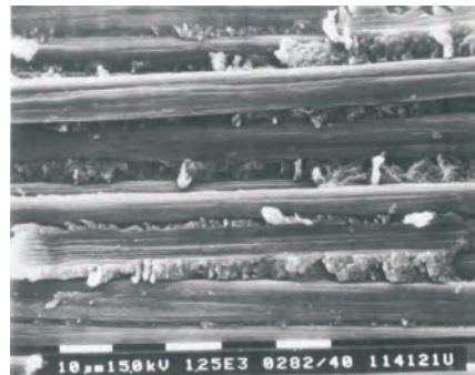
(f) Mode II delamination in wet specimen of T300/914C. Moisture content is 2.53%
