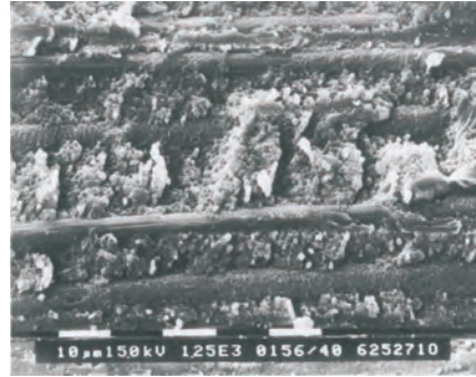
(b) Mode II delamination in wet specimen of T300/M21. Moisture content is 0%
