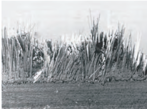
Figure 1.2: SEM image with a broom-like tension failure of a GFRP laminate [46].
