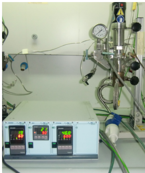
Figure 3.5-1: Catalytic activity test setup used for the hydrogenolysis of glycidol.
