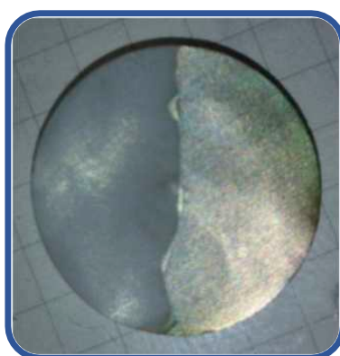
Figure II-16. PTFE sample coated with metallic silver. Two areas can be differentiated, a non-modified one (left) and the coated with silver (right). The plasma power peak was set at 15 W with a DC of 0.5 with PFM for 3 min. After the plasma, there was a 3 min of PFM flow and then samples were incubated with 3 mL of glucosamine 1 M for 5 h, and then washed with Milli-Q water. Finally, samples were incubated with Tollens' reagent (1 mL \text{AgNO}_3 1 M + 2 x 25 \mu\text{L} \text{NH}_3 , 15%) for 60 min at 90°C.
