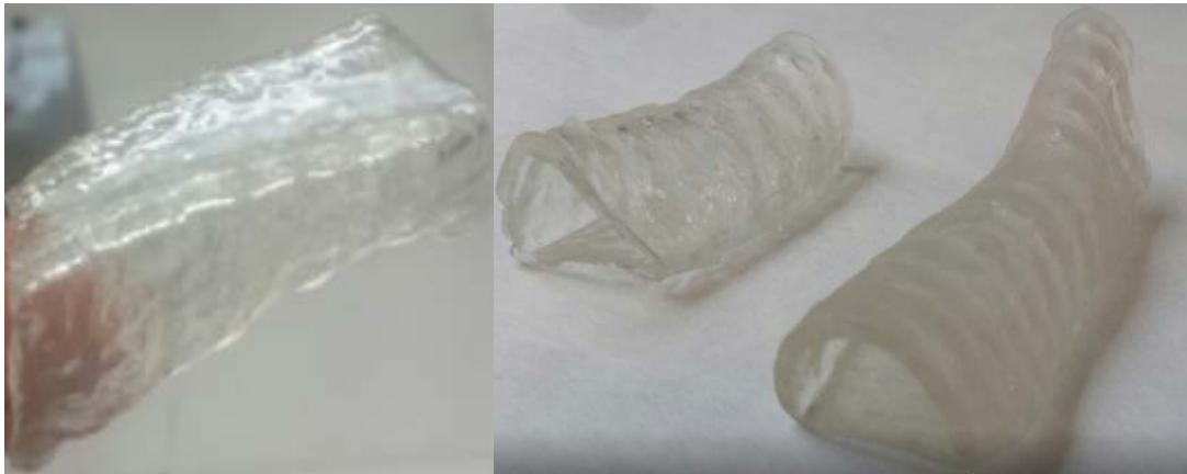
Figure IV-17. Anatomical silicone stents manufactured using 3D printing technology in combination with mould fabrication.
