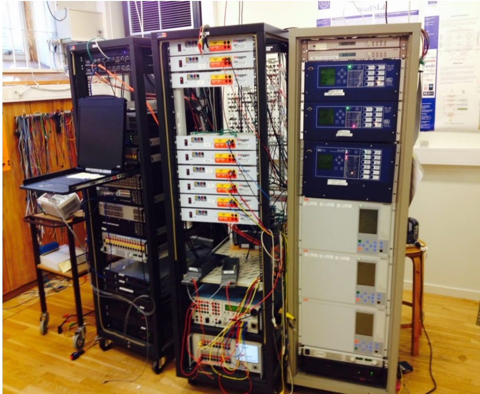
Fig. A.2. The HIL test-bed (SmarTS Lab, KTH University)
