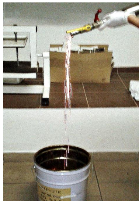
Fig. 5.2 nZVI pyrophoricity tests.
