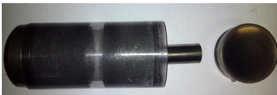
Fig. 5.18 Polycarbonate vial, caps and smashing cylinder.
