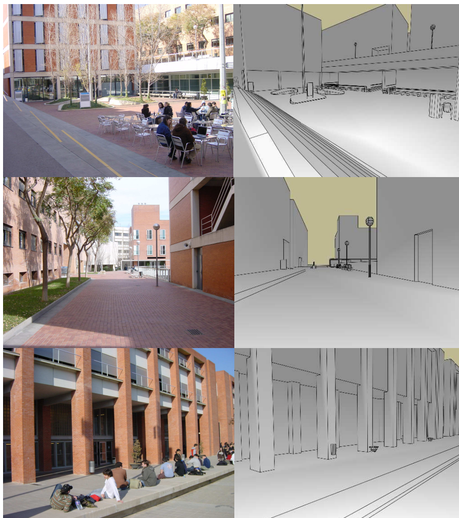
Figure 4.3: Pictures of the UPC campus environment and their approximate corresponding snapshots of the 3D map. The 3D map is static and only models the most significant parts of the environment.
