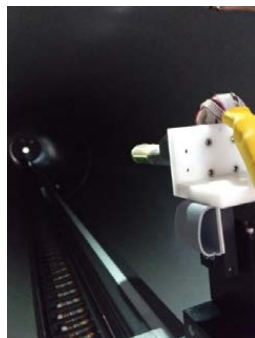
Figure 1: Boom mounted inside the tunnel
