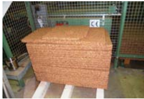
(a) Cork granulated-agglomerated insulating panel (end product)
