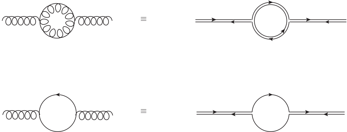
Figure 4.1: Feynman diagrams for the LO contribution to the gluon self-energy: using the usual notation (left), and with the double line one (right).
